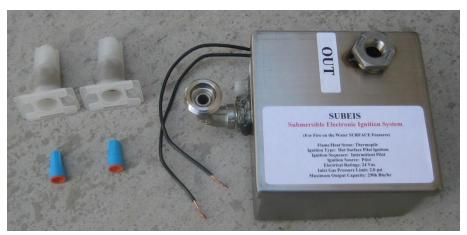
Electrical Connections – to ensure a watertight electrical connection we have provided you two DRYCONN waterproof connectors (blue and orange wire nuts in photo) along with two DRYCONN Grease filled Strain Relief (Opaque Connectors above wire nuts). We recommend using both for maximum waterproof protection.
