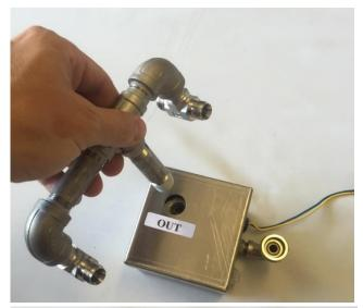
The first step to installing the Submersible Manifold is to install the part of the manifold that threads into the outlet of the SUBEIS.
