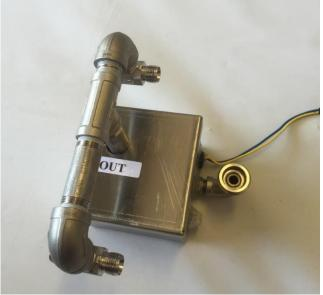
The photo at left shows what this step looks like once complete. Notice the fittings are perpendicular to the sides of the SUBEIS Ignition Control Box.
